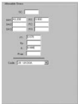
**Figure 15 - CAESAR II Allowable Stress Auxiliary Data Screen (UKOOA)**
