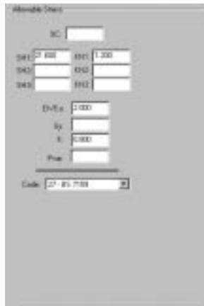
**FIGURE 14 - CAESAR II Allowable Stress Auxiliary Data Screen (BS 7159)**
